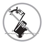
Use extreme care and slow speeds while driving the machine in the stowed position across uneven terrain, debris, unstable or slippery surfaces and near holes and drop-offs.
