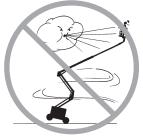
Do not raise the boom when wind speeds may exceed 28 mph / 12.5 m/s. If wind speeds exceed 28 mph / 12.5 m/s when the boom is raised, lower the boom and do not continue to operate the machine.
