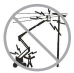
Keep away from the machine if it contacts energized power lines. Personnel on the ground or in the platform must not touch or operate the machine until energized power lines are shut off.
